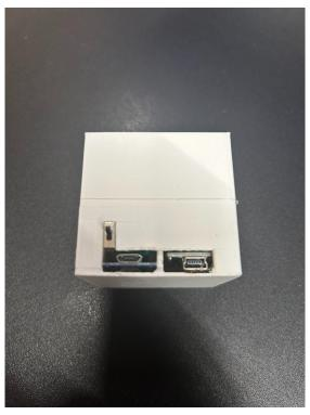
The last step is to use super glue to attach the top and bottom pieces of the enclosure together.
