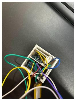
The 3D printed enclosure allows for both the nano and the charging circuit to be housed tightly in the cube, with USB's facing outward and accessible. I used hot glue to glue them down to the enclosure as well. I have the pins for the nano facing upwards. There is storage too for the battery to fit in.
