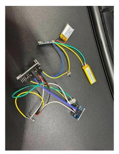
Put the circuit together. Remember to always use a breadboard first before soldering to ensure everything is working correctly. Note I am using two 3.7v lipo batteries in parallel. This is not good practice, but shouldn't cause much of an issue. Never attach batteries in series to a charging circuit.
