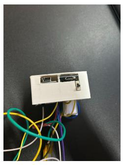
I then used super glue to carefully glue the switch into the little slot on the enclosure. If you have a bigger switch, you can dremel out the slot to accommodate it.
