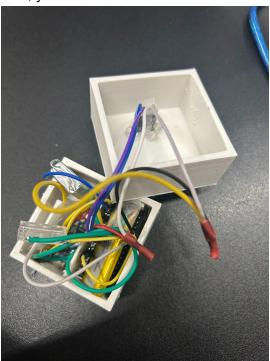
The next step is to feed the OLED wires through the slit on the top part of the housing, and hot glue it in place (the device will be shaken, so glue it well).
