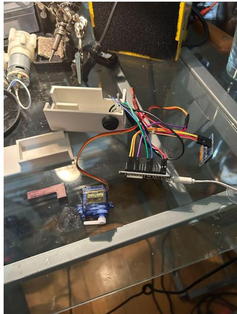
Once the circuit and code are good to go, unplug the USB power and disconnect the OLED screen (you will need to feed wires through the slot at the front). Insert the NodeMCU upside down into the configured slot like this, it should be a snug fit. Re-connect the OLED after pushing the wires through the slot in the front. Attach the PSU to the NodeMCU and test that everything is working and ready to complete.
