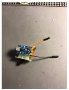
The first thing to do is to create a lipo charging circuit with on/off switch. Full instructions can be found under the "projects" tab on my website yokon.net/lipocharger. This is also shown in the circuit diagram above.
