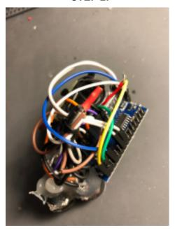
Complete the circuit in the diagram above. Since theres only 1 GND port available on the nano (other than the one for the PSU), so the solution is to twist all the components ground wires into 1 and solder it together. The group of cables with the red heat shrink tubing is the ground cable joint.
