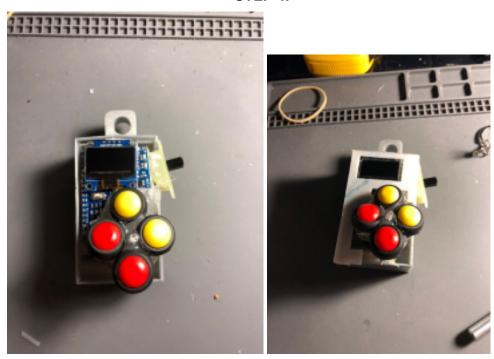
Place the glued circuit in the case, glue the top down ontop.
